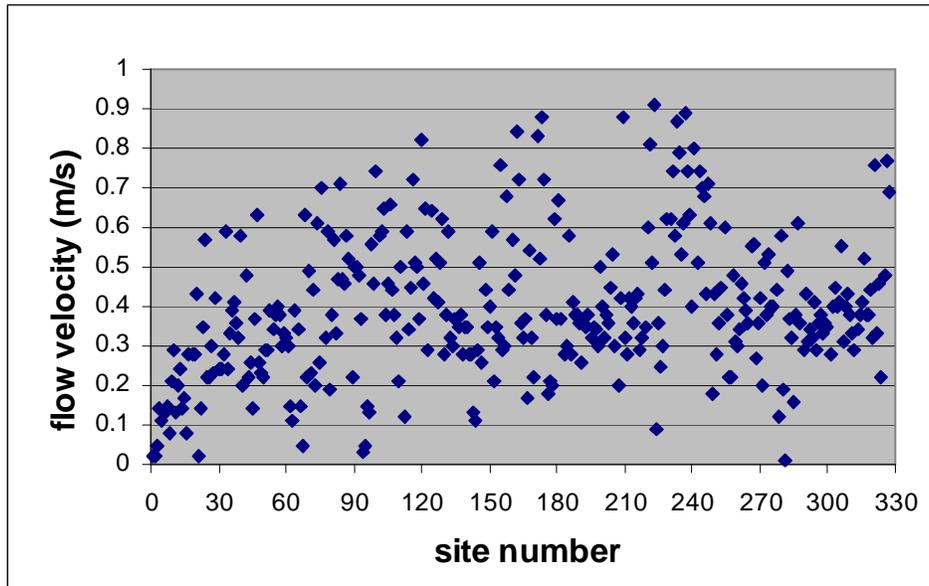
**Figure 6 Flow velocity (@ 80%) profile of the Namekagon River at thalweg**
