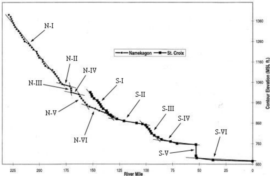
**Figure 2 Major segments of Macbeth *et al.* (1999)** The X-axis is river mile upstream from the confluence of the St. Croix River and the Mississippi River. The Y-axis is the elevation. *Major Segments* on the St. Croix River and the Namekagon River are denoted by “S” and “N” separately.
